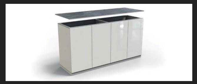
Worktops must be attached to cabinets with silicone sealant. Due to their thickness, screws are not suitable for fixing these surfaces. Silicone should be applied at a distance of 10 mm from the front edge of the body.
