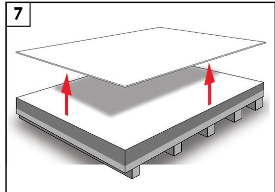
7. The production shall be carried out in such a way that friction between two panels is eliminated in order to protect the surface.
