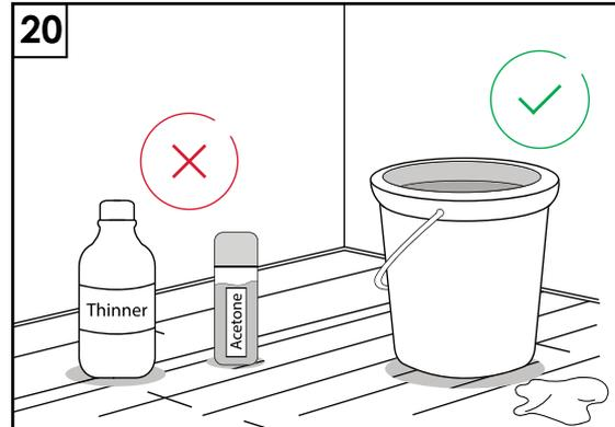
20. Wet-cotton cloth, soapy-cotton cloth or alcohol-free fluid surface cleaning agents shall be used for cleaning the products. Alcoholic surface cleaning agents and scrubbing agents shall never be used. When you use such agents, it will cause tarnishing and scratching on the surface. Thinner and substances that contain acid shall never be used for cleaning.
