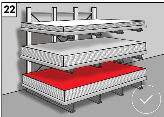
22. Pallets shall be stowed by placing them on shelves or on level area in such a way that maximum 4 pallets are put on the top of each other.
