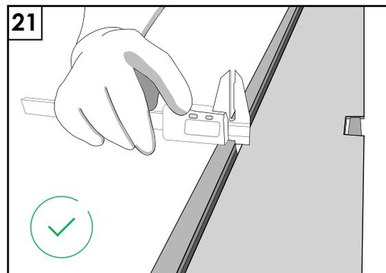
21. The extent of rotation on the panel shall be 4mm for shorter edge and maximum 10 mm for the taller edge. This tolerance may vary for the topmost sheet since it is reversed. After the panels are dimensioned rotation values fall within useable tolerance limits.
