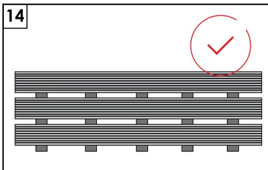
15. When panels are put into process stowing shall be applied cautiously in order to prevent the formation of crushing, collapse and fracture at the edges and corners.
