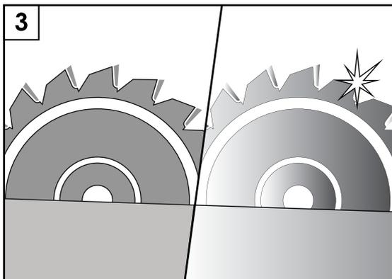
3. It shall be ensured that the saw is ground well.
