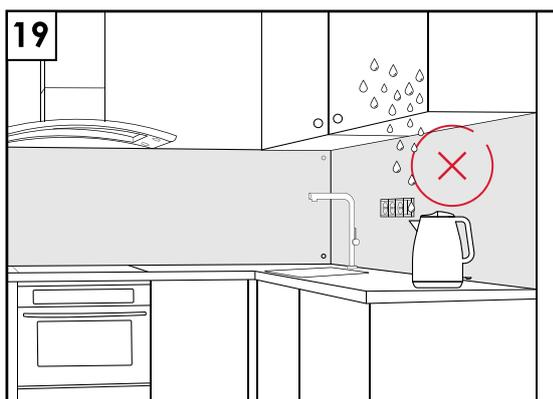
19. Products shall not be used at the open spaces, gardens and places where are washed through water and where are directly subjected to steam.
