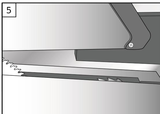
5. In order to obtain better results, jumping saw with scriber shall be used for panel cutting.
