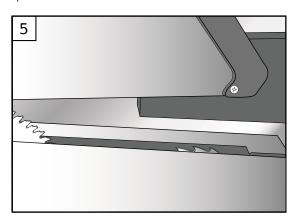
5. In order to obtain better results, jumping saw with scriber shall be used for panel cutting.
