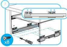
Align lower runners flush under metal plates. Drill and screw lower runners.
