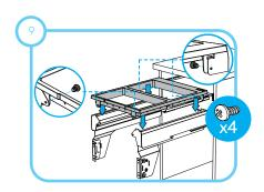
Install plastic tray loosely with screws, allowing for adjustment.
