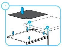
Adjust metal tray position, tighten screws when parallel. Place mat on top.
