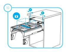
Adjust plastic tray position, tighten screws when parallel.
