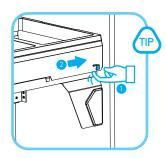
To release brackets from the runners, click swit**ch** 1 on the sides of the brackets and slide out 2
