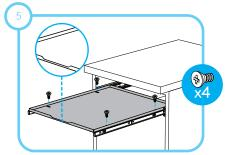
Install metal tray loosely with screws, allowing for adjustment.
