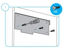
Attach both left and right metal plates to cabinet wall using supplied screws.
